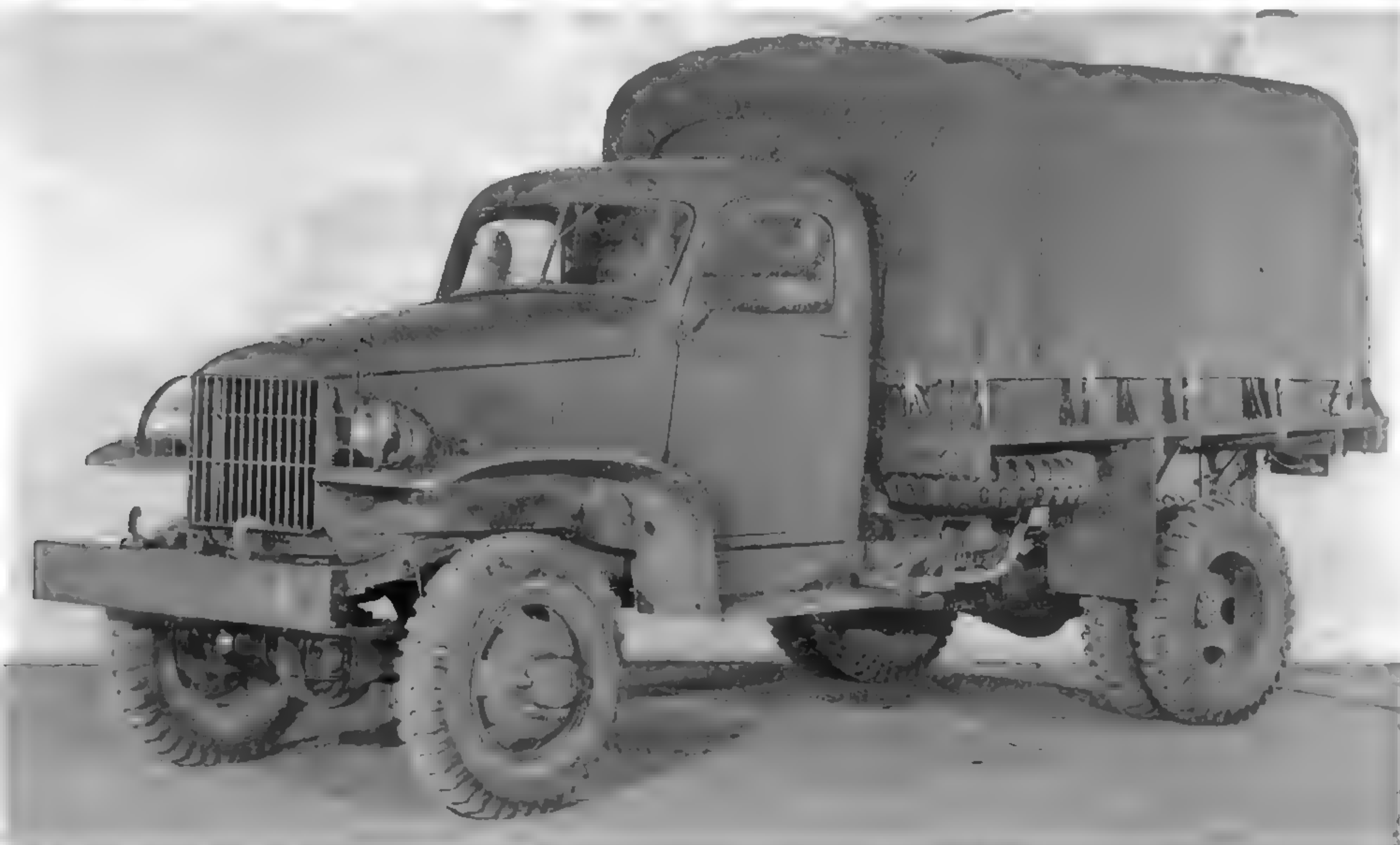
This Army Engineering Standards Vehicle Laboratory photo taken in January 1944 shows a G7107 with the canvas bed cover. The cargo bed on this truck is made of wood. The stenciling on the side of the canvas indicates it was made for the U.S. Q. M. C. (U.S. Quartermaster Corps), although the maker's name is not legible. (U.S. Army photo)
